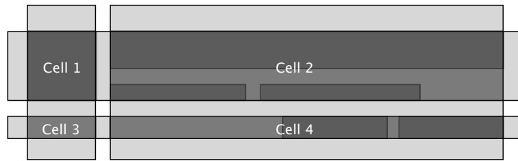
Figure 3.1: The row and column grouping applied on the interface from Figure 2.1. The dark shades of gray are the original bounding rectangles (frames) of the interface elements. The light shades of gray represent rows and columns. The intersections of rows and columns are the cells.
